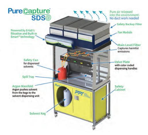
PureCapture™ SDS integrated with Erlab's advanced filtration, detection and communication, allows Pure Process Technology to provide a completely independent SDS system without the need for any facility HVAC.
