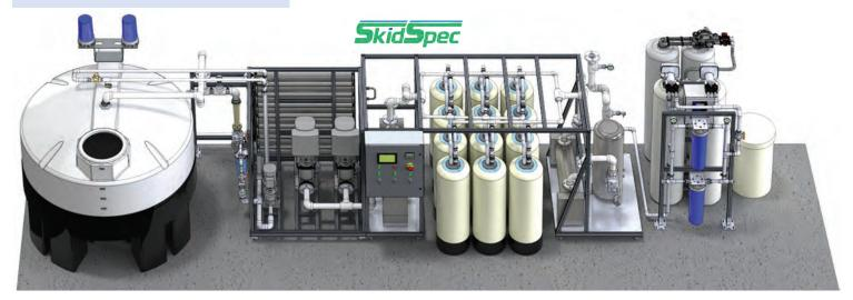
This drawing incorporates all options available, with PPT's high quality components, for building an RO/DI high purity water system.
